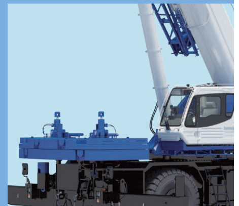
Counterweight mounting/dismounting cylinder
