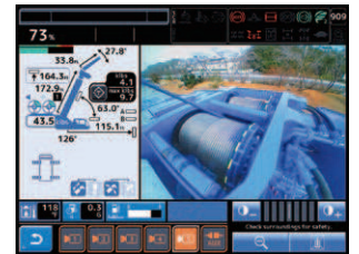
Winch drum monitoring camera * The camera image in the photo are simulated.
